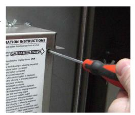
4. Release the calibration button when the totaliser display shows **VER** followed by the version number on the lower line of the display.
