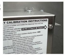
3. Gently push and hold the calibration button using a small screwdriver or similar tool.
