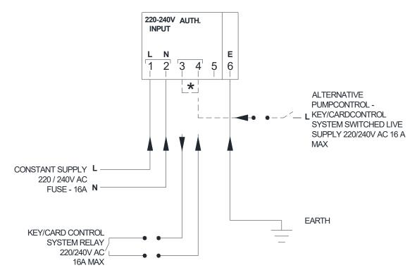
★ SUPPLIED WITH LINK FITTED BETWEEN TERMINALS 3 AND 4. REMOVE LINK FOR REMOTE KEY/CARD CONTROL
