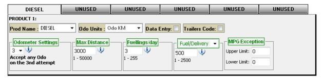
Up to six products can be assigned to a Tag on the fuel control system. To assign a fuel type select the first unused option on the top of the screen.
